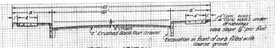
Note: 6" concrete base to be applied under sidewalks to be applied under them. All street material walks to be applied under sidewalks.
