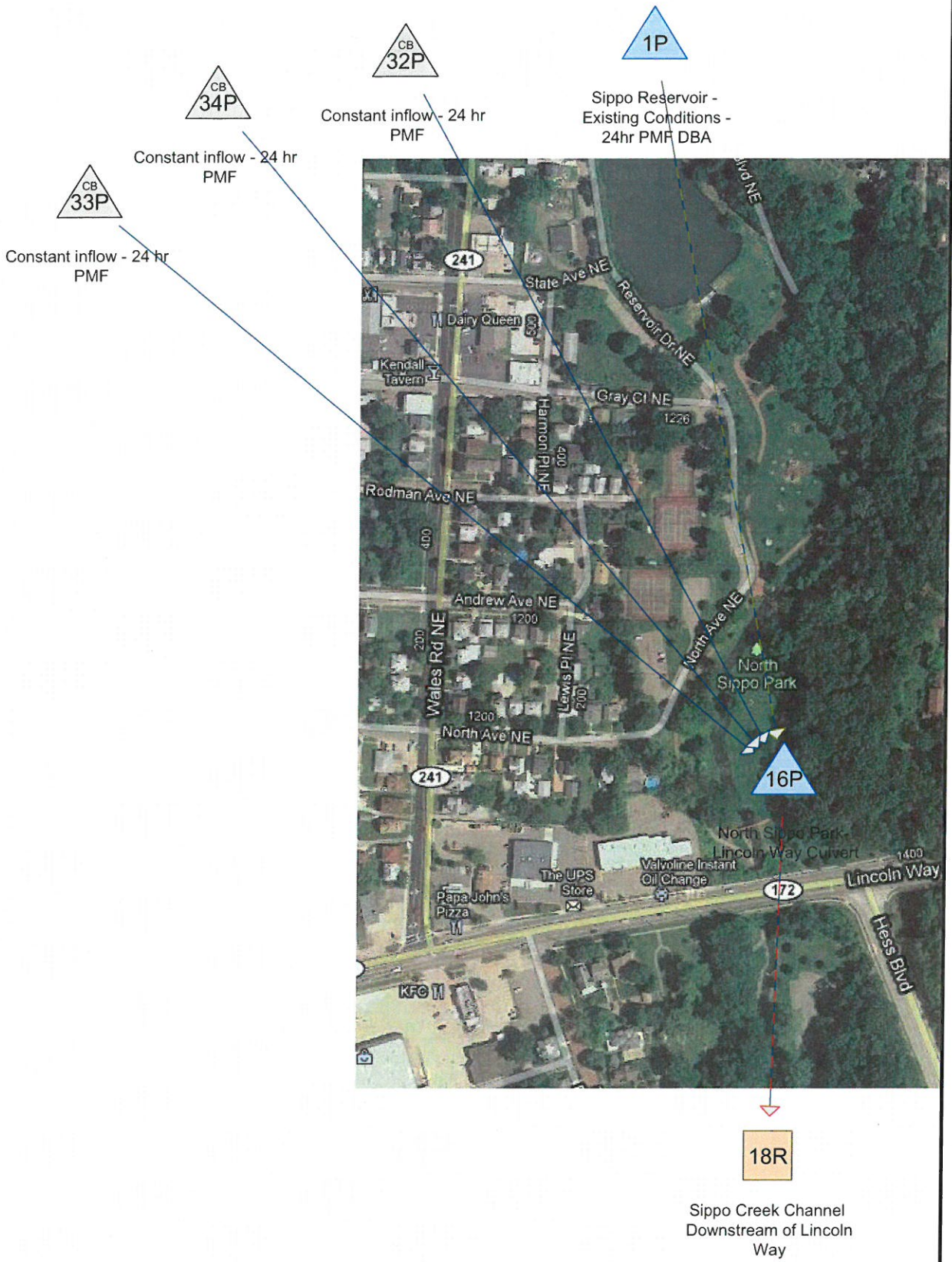
Drainage Diagram for Existing Conditions Sippo Reservoir-URS-DBA-24-hrPMF Prepared by URS Corporation, Printed 10/31/2011 HydroCAD® 9.10 s/n 04378 © 2010 HydroCAD Software Solutions LLC
