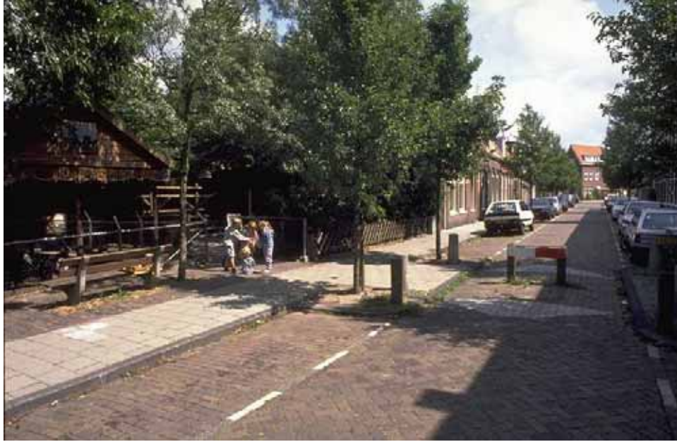
Figure 20-13. Photo. The design of street closures should provide specific parking areas to discourage obstruction of bicycle and pedestrian traffic.
