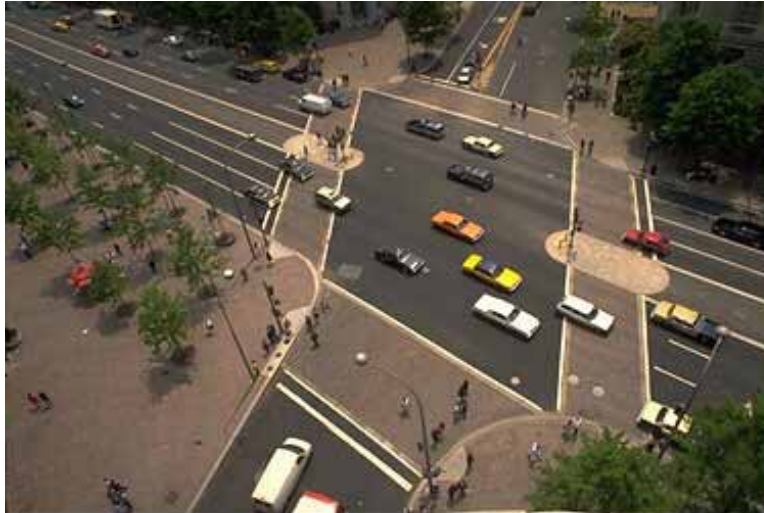
Figure 11-2. Photo. Use of colored crosswalks and median refuges makes this intersection more pedestrian-friendly.
