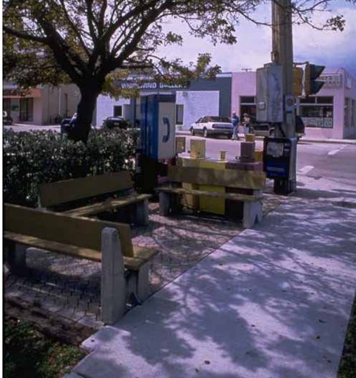
Figure 9-5. Photo. This corner features public telephones and a sitting area that does not encroach on the walkway.
