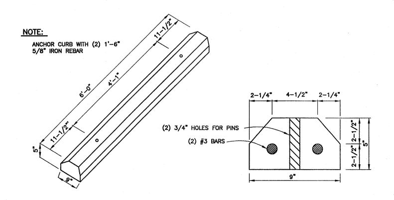
TYPICAL PRECAST PARKING CURB STOP DETAIL
