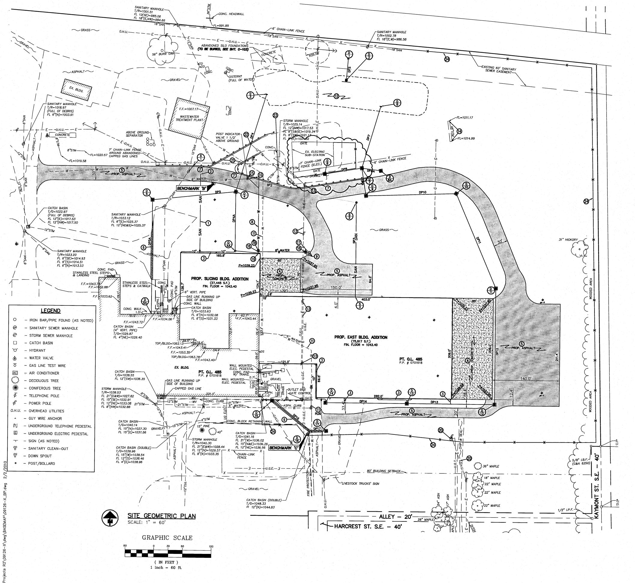
BENCHMARK 'B': TOP OPERATING NUT OF HYDRANT LOCATED APPROX. 160' N. OF THE PROP. BUILDING ADDITION
