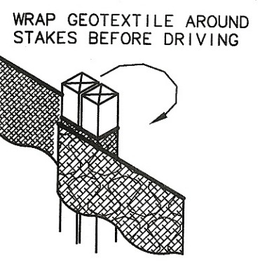
JOINING SECTIONS OF SILT FENCE DETAIL NO SCALE
