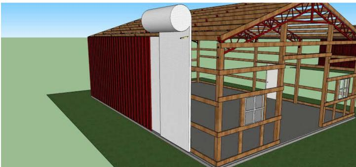
Attach eave trim on top of eave strut, hanging over top of sidewall panel. Add inside closure and butyl atop eave trim.
