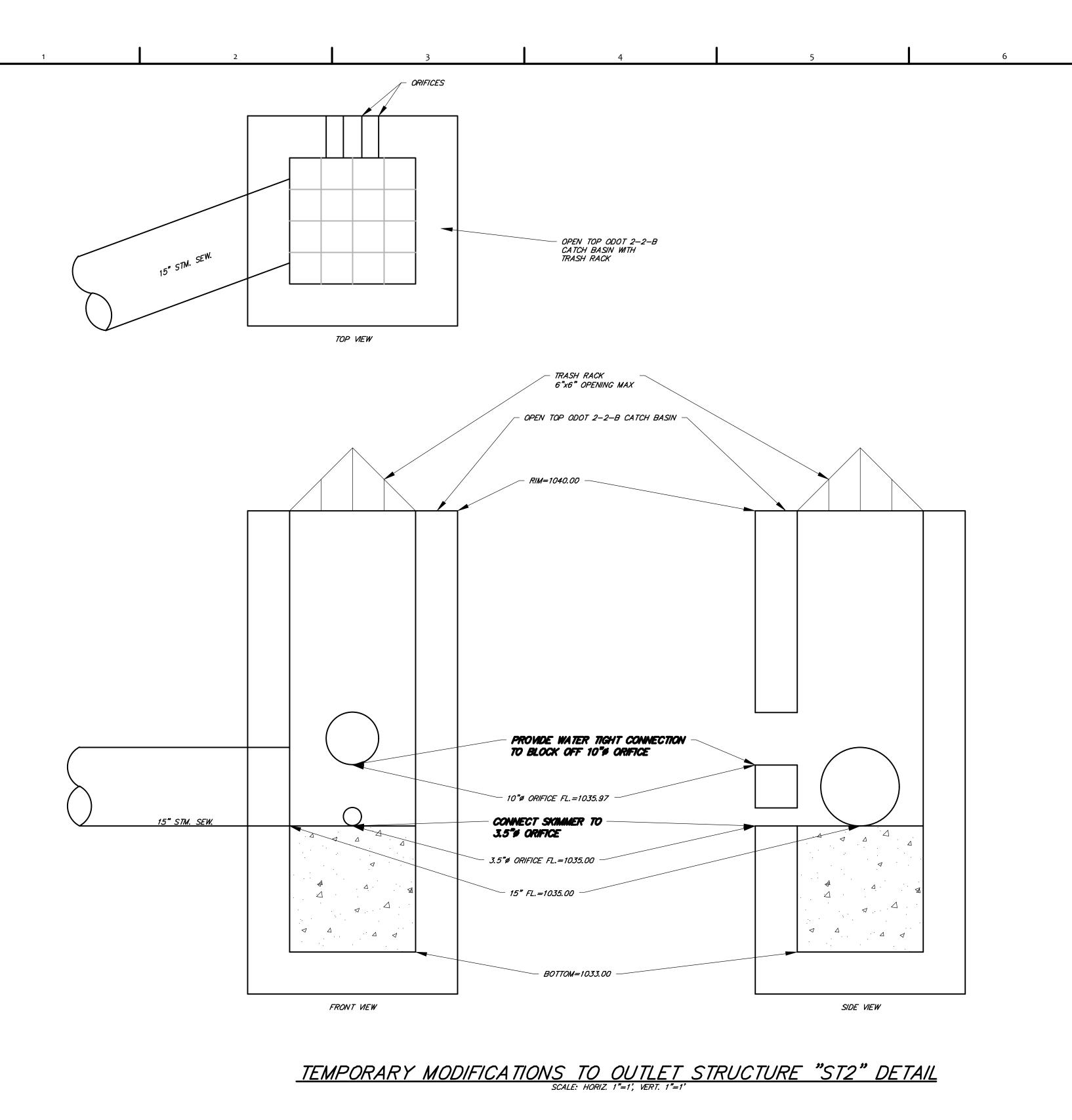
SEDIMENT BASIN NOTES: THE PROPOSED STORMWATER MANAGEMENT BASIN SHALL BE USED AS A SEDIMENT BASIN DURING CONSTRUCTION. DURING ITS USE AS A SEDIMENT BASIN THE FOLLOWING OPERATION AND MAINTENANCE SHALL BE ADHERED
