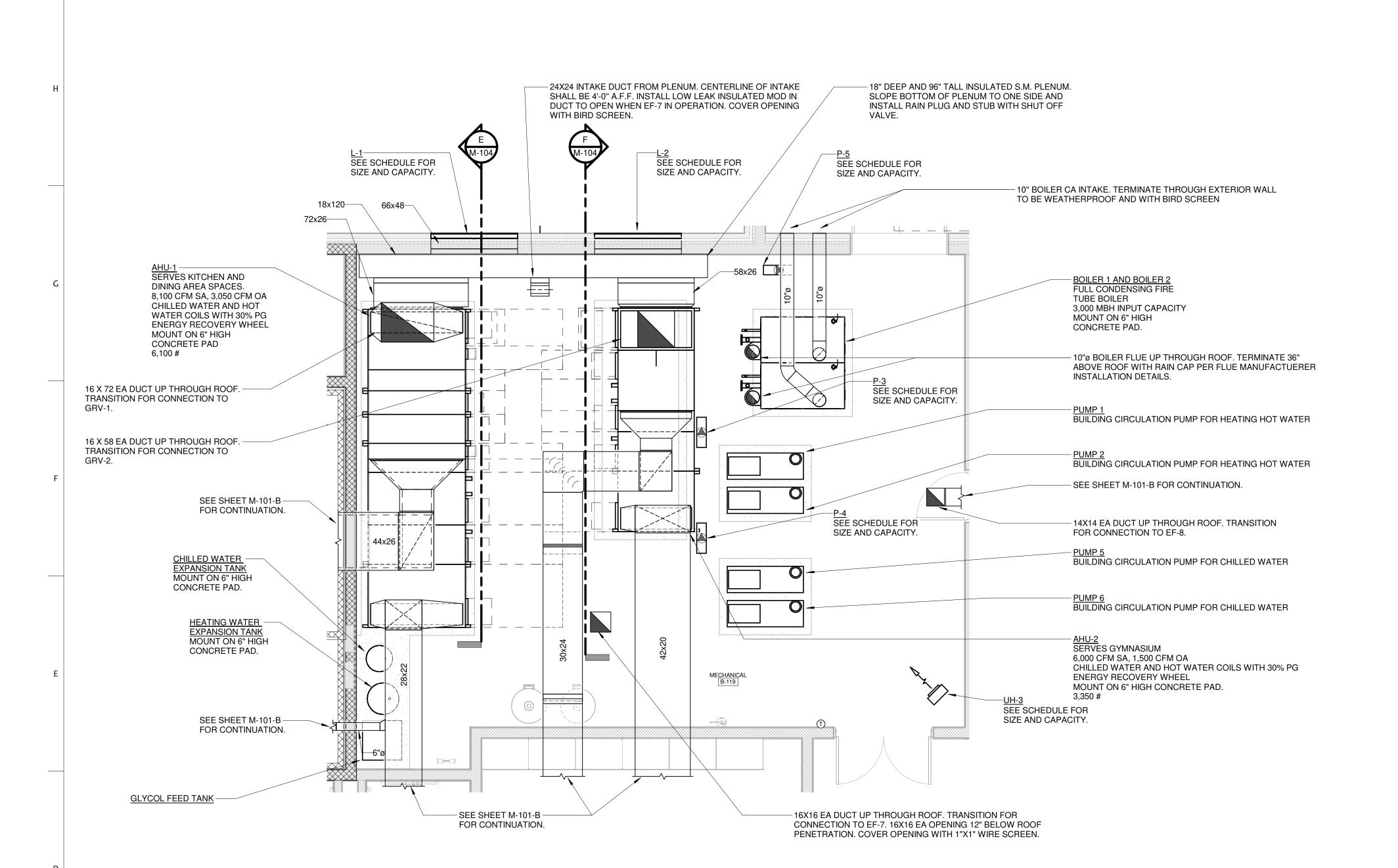
PARTIAL FIRST FLOOR PLAN - ENLARGED MECH ROOM B-119 - HVAC
