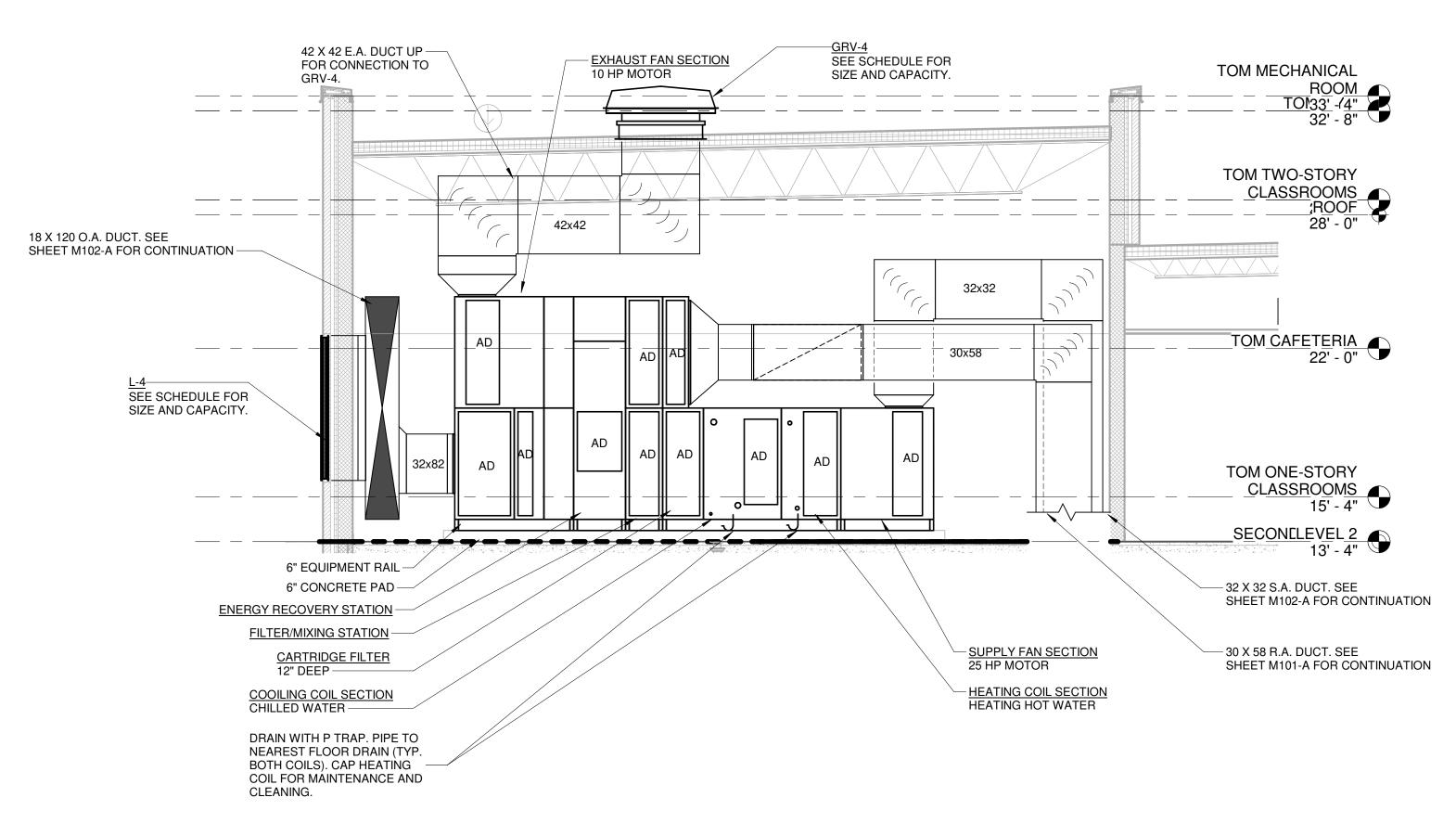
Section D-D (AHU-4 MR A-229) SCALE: 1/4" = 1'-0"
