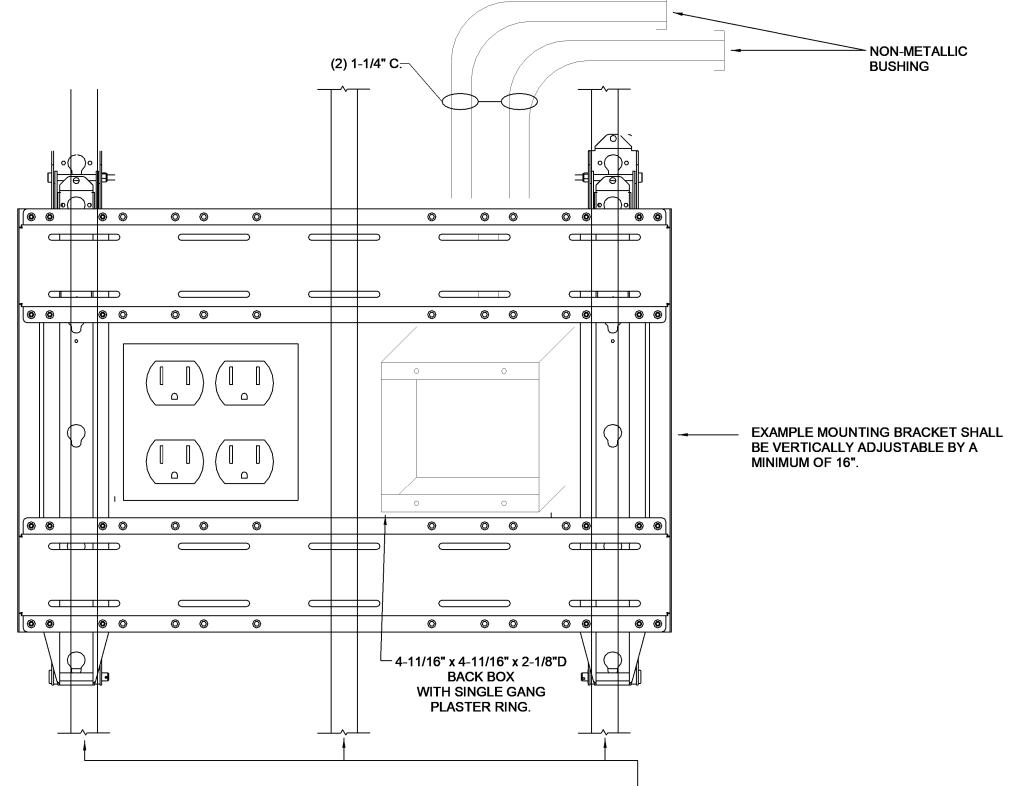
STANDARD WALLSTUDS ON 16" CENTER. ALIGN WALL MOUNT WITH MOUNTING -HOLES AND STUDS PER MANUFACTURERS RECOMMENDATION. PROVIDE BACKING AS NECESSARY. COORDINATE HEIGHT WITH ARCHITECTURAL ELEVATIONS.
