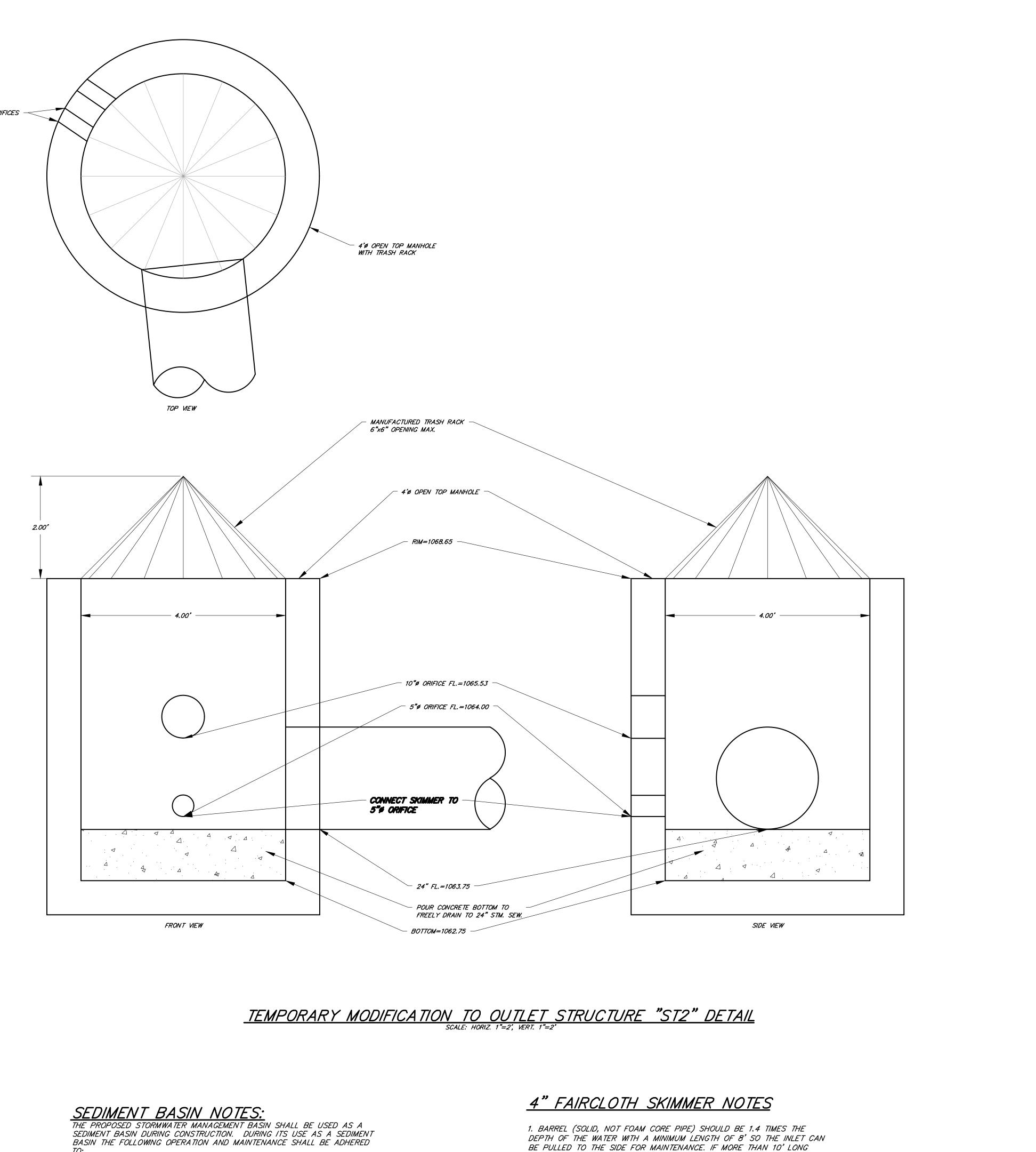
1. CONTRACTOR SHALL MODIFY STORMWATER MANAGEMENT BASIN AS DEPICTED ON THIS SHEET AS A TEMPORARY SEDIMENT BASIN UNTIL CONSTRUCTION IS COMPLETED AND UPLAND AREAS ARE STABILIZED. 2. FAIRCLOTH SKIMMER SHALL BE INSTALLED AND MAINTAINED WHILE SITE IS UNDER CONSTRUCTION.
