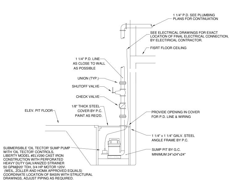
ELEVATOR PIT SUMP PUMP DETAIL
