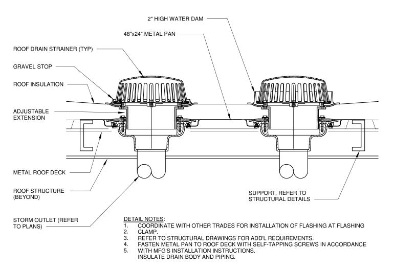
STORM AND OVERFLOW ROOF DRAIN DETAIL
