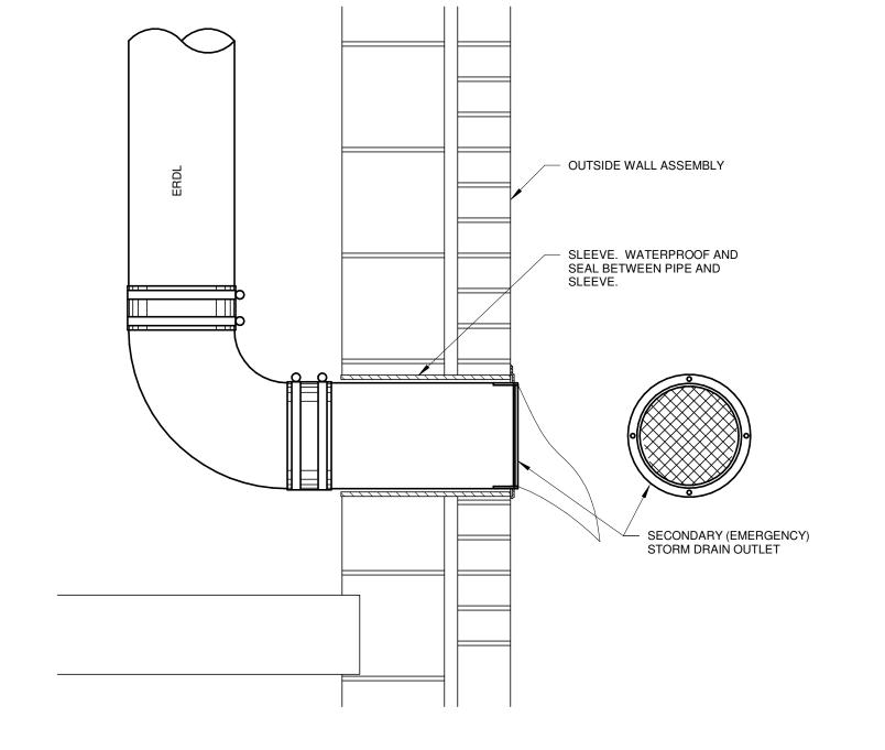
EMERGENCY STORM DRAIN OUTLET DETAIL
