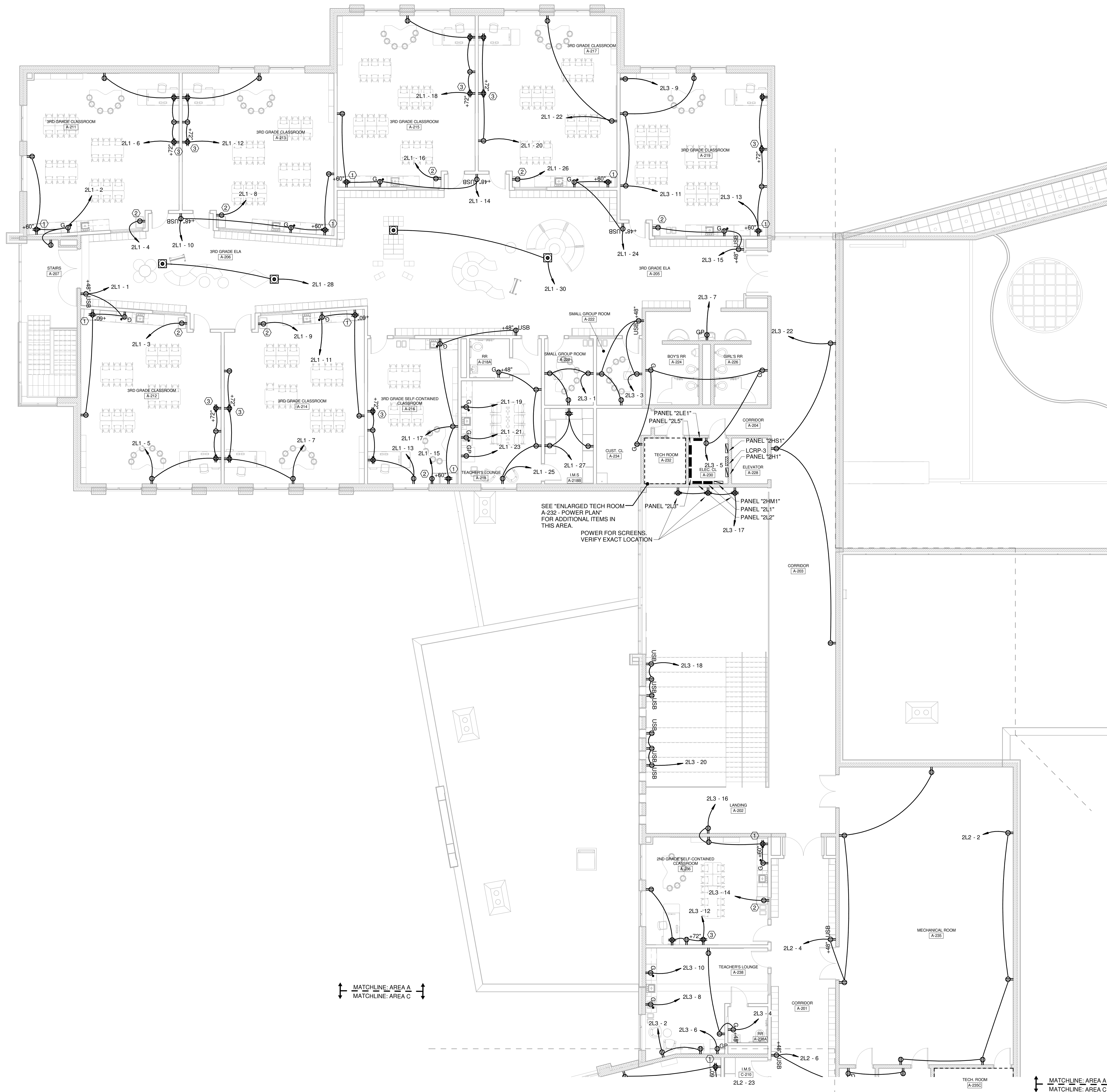
ENLARGED TECH ROOM A-235C - POWER SCALE: 1/4" = 1'-0"
