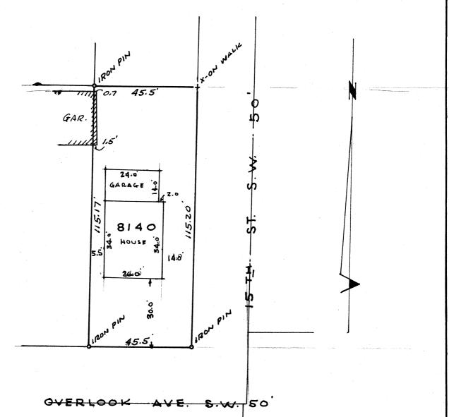
THE ABOVE PROPERTY IS LOCATED AT 821 15 TH ST. S.W. MASSILLON, OHIO, I HERE BY CERTIFY THAT THIS SURVEY SHOWS THE IMPROVEMENTS ARE LOCATED ON THE PREMISES DESCRIBED, THAT ALL DIMENSIONS SHOWN HEREON ARE CORRECT, THAT THE IMPROVEMENTS ARE BUTIRELY WITHIN THE LOT LINE LIMITS AND THE ONLY ENCROACH MENT IS THE GARAGE ON THE WEST SIDE OF SAID LOT NO 8140 AND THERE THE DARE NO OTHER ENCROACH MENTS FROM ADJOINING PREMISES.
