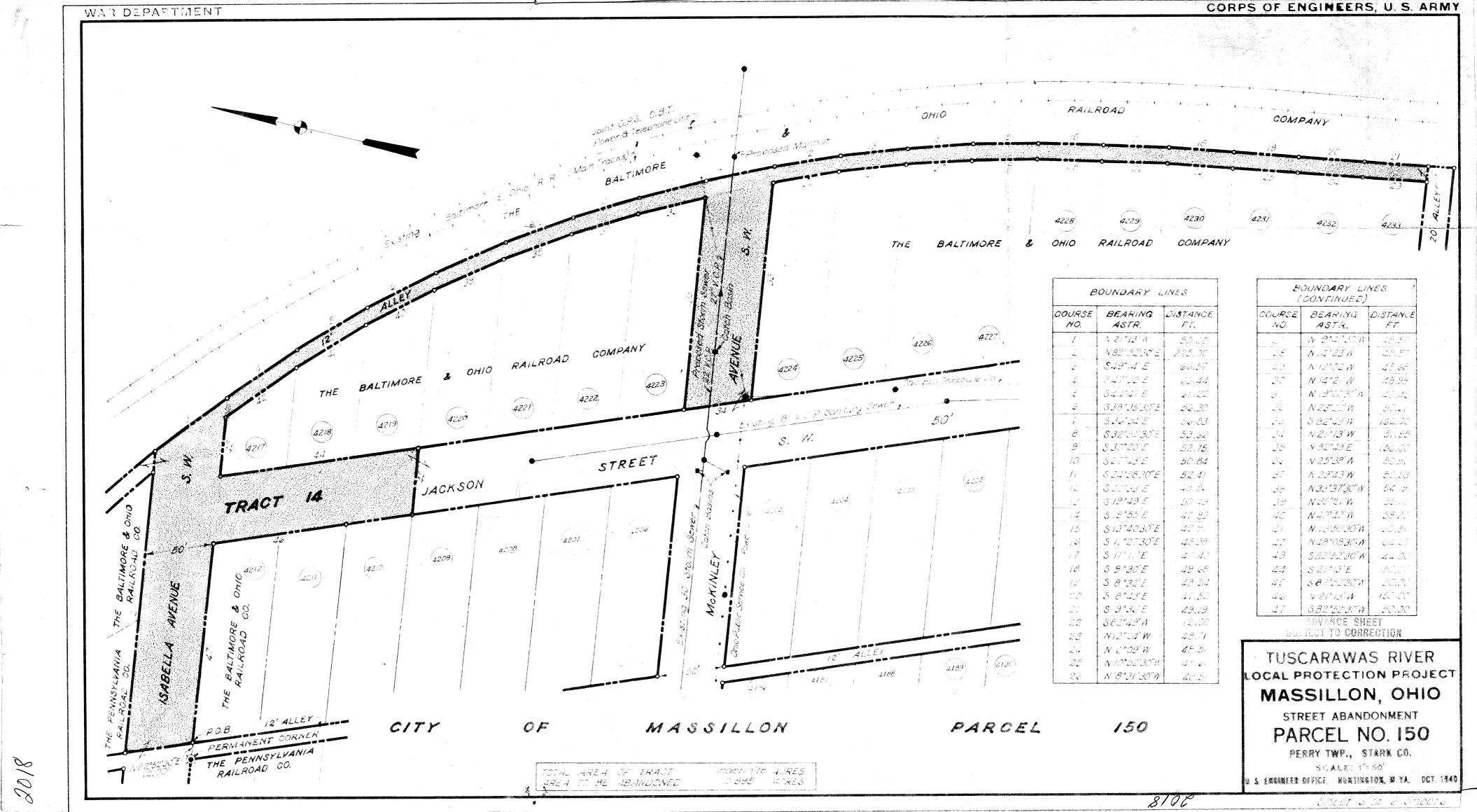
thence, from the said point of beginning, S 31° 17' E, 305.95 feet, to a point in the eastern boundary line of the right of way of The Pennsylvania Railroad Company; thence, along this boundary line, N 52° 10' 30" W, 108.20 feet, to its intersection with the said western boundary line of Third Street S.W.; thence, along the last mentioned boundary line, N 20° 37' W, 208.47 feet, to the point of beginning; containing 0.137 acre, more or less.
