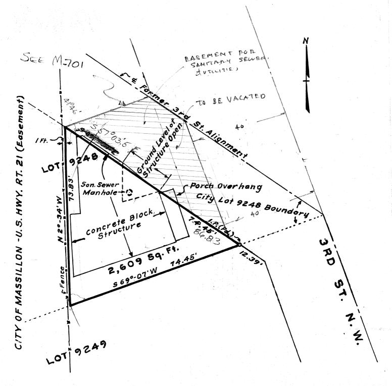
DRAWING OF THE PART OF LOT 9248 LYING EAST OF U.S. RT. 21 SHOWING LOCATION OF BLOCK STRUCTURE IN CITY OF MASSILLON STARK COUNTY, OHIO.
